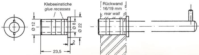
**MINI 8 with collar (front) for gluing**
